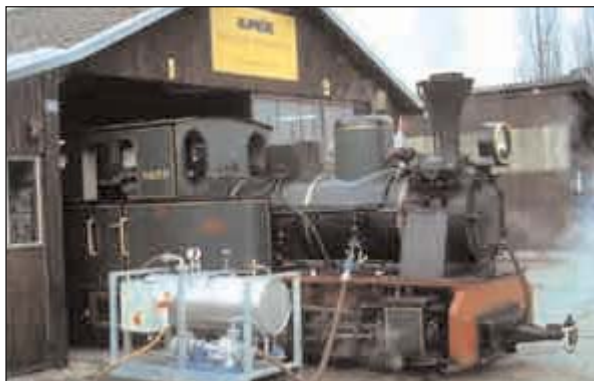
Fig. 8: The electric preheating device can also be used for coal-fired steam locomotives, considerably reducing the amount of smoke produced during lighting up. Neighbours are delighted.
