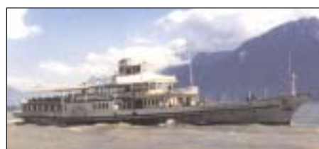
Fig. 24: The "Montreux" after conversion to diesel-electric drive, which improved the economics but certainly not the aesthetics.
