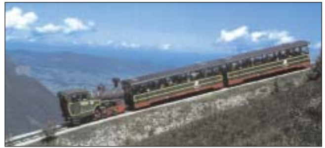
Fig. 14: Locomotive No. 999.201 of the Schafberg Railway with a full load of passengers on 1 in 4 grade. Note the clean combustion at full load.
