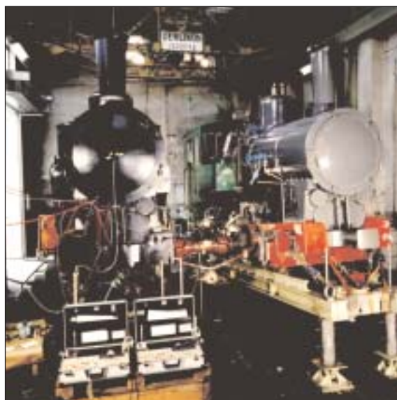
Fig. 10: Work load trials at SLM with locomotive No.12 of the Brienz-Rothorn Railway on the left side and 999.201 of the Austrian Federal Railway. The two bright cases in the foreground contain the emission analysers.
